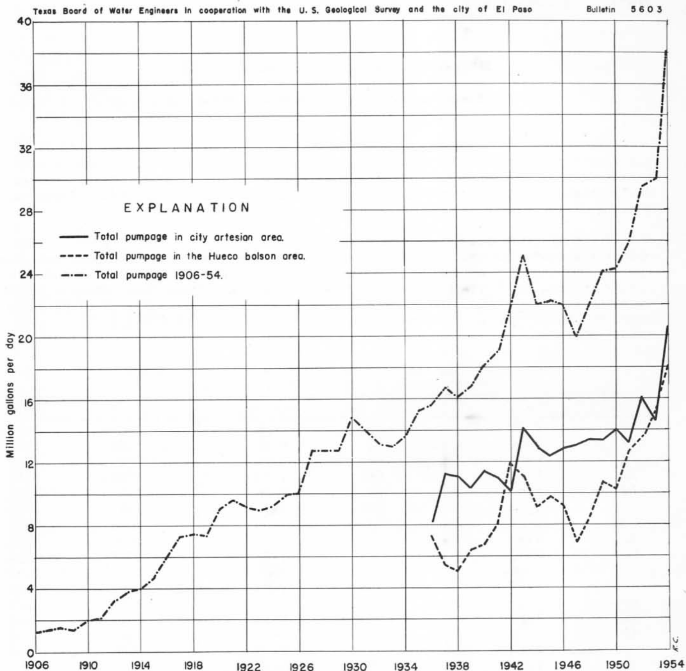
FIGURE 1.—Average daily pumpage from all deep wells in the Hueco bolson and city artesian areas, 1906-54.
