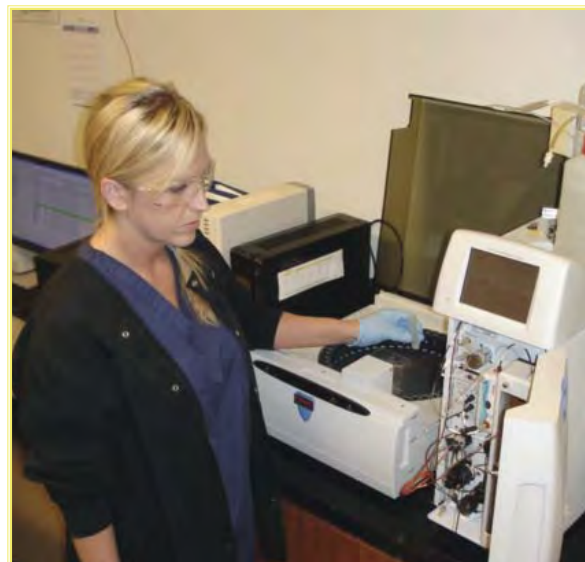
Thermoscientific 2100 Ion Chromatograph
