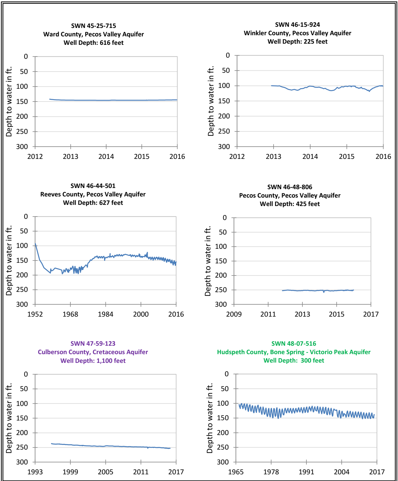
Figure 4-2 (continued) Hydrographs of TWDB recorder wells in West Texas. Undesignated or local aquifer indicated in purple text. Minor aquifers indicated in green text . SWN = state well number
