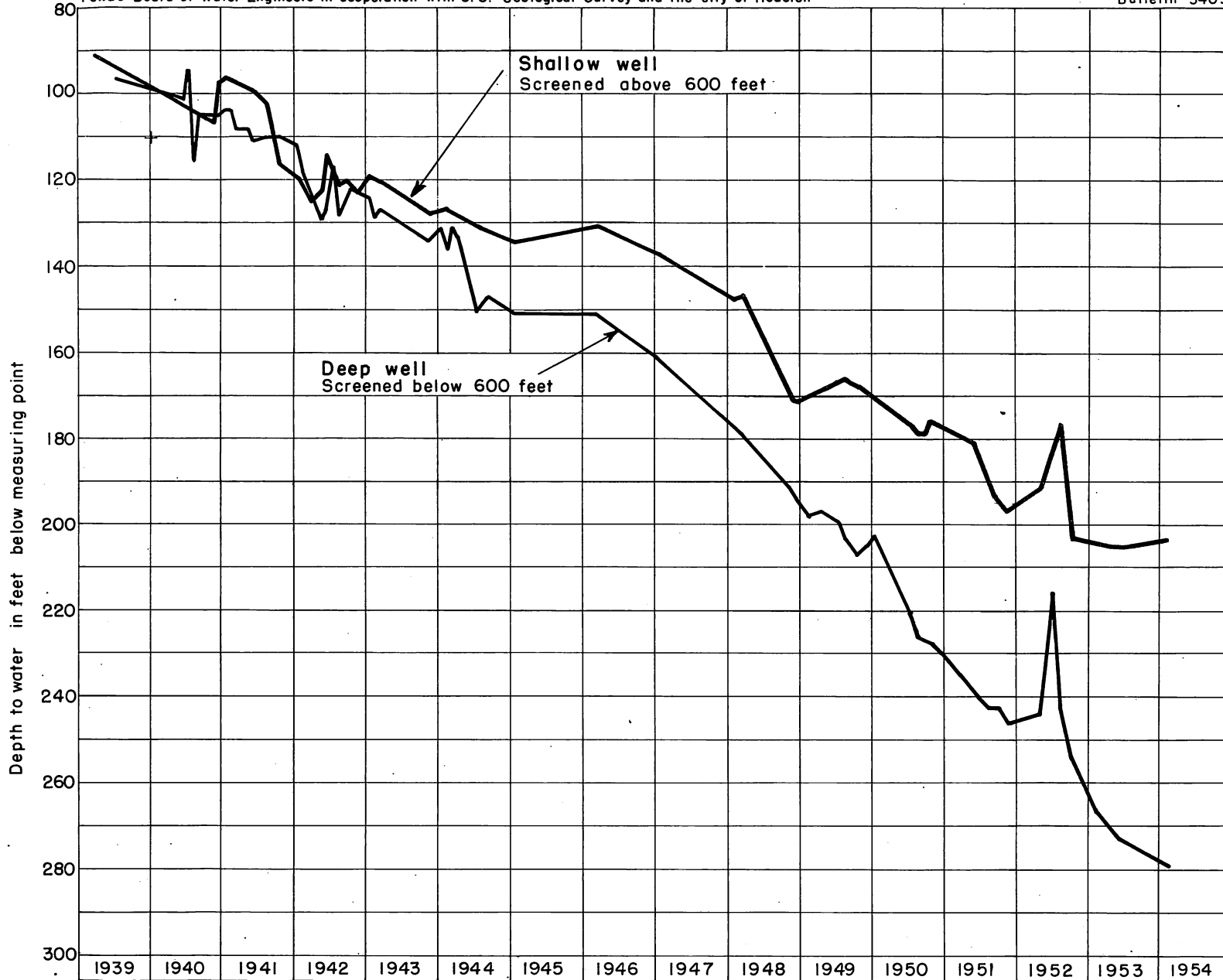
FIGURE II.- Comparison of declines of artesian pressure in a shallow well and a deep well in the eastern Ship Channel-Pasadena area, Texas.
