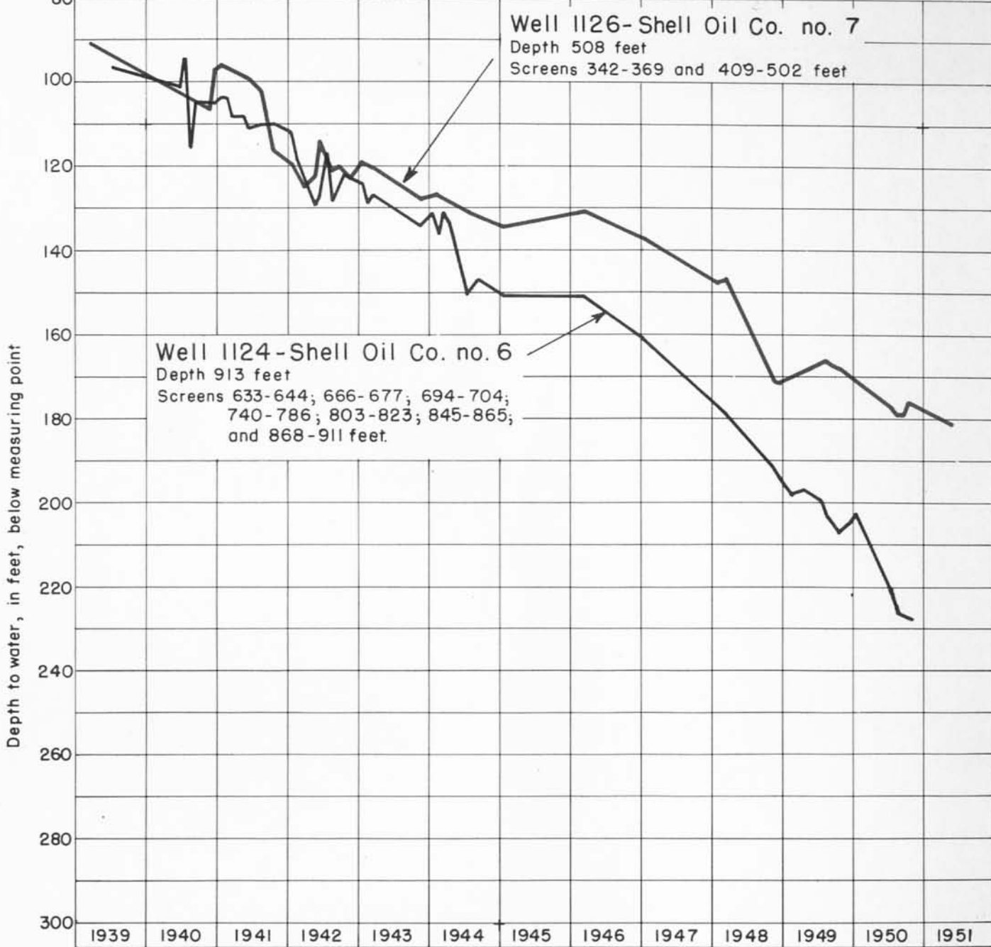
FIGURE 9.- Comparison of declines of artesian pressure in a shallow well and a deep well in the eastern Ship Channel-Pasadena area, Tex.
