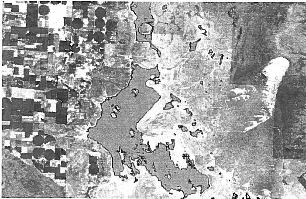
Figure 10. Playa zones on the July 4, 1985 TM data differentiated at a band 5 threshold reflectance level of approximately 0.30. Dunes constitute the features to the right of the large ca. 16 square mile playa area shown. Irrigated acreage surrounding Dell City is visible to the left.
