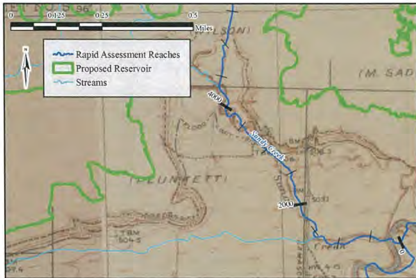
Figure 5.40 - Comparison of Historic to Existing Channel Alignment on Sandy Creek.
