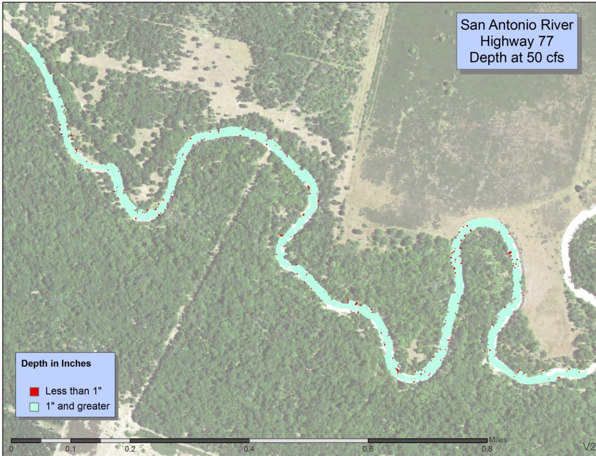
Figure H-5. Spatial output of longitudinal connectivity at the simulated flow of 50 cfs for the San Antonio River Hwy 77 Study Site.
