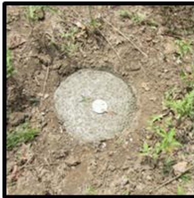
Figure 11. Typical survey reference mark.
