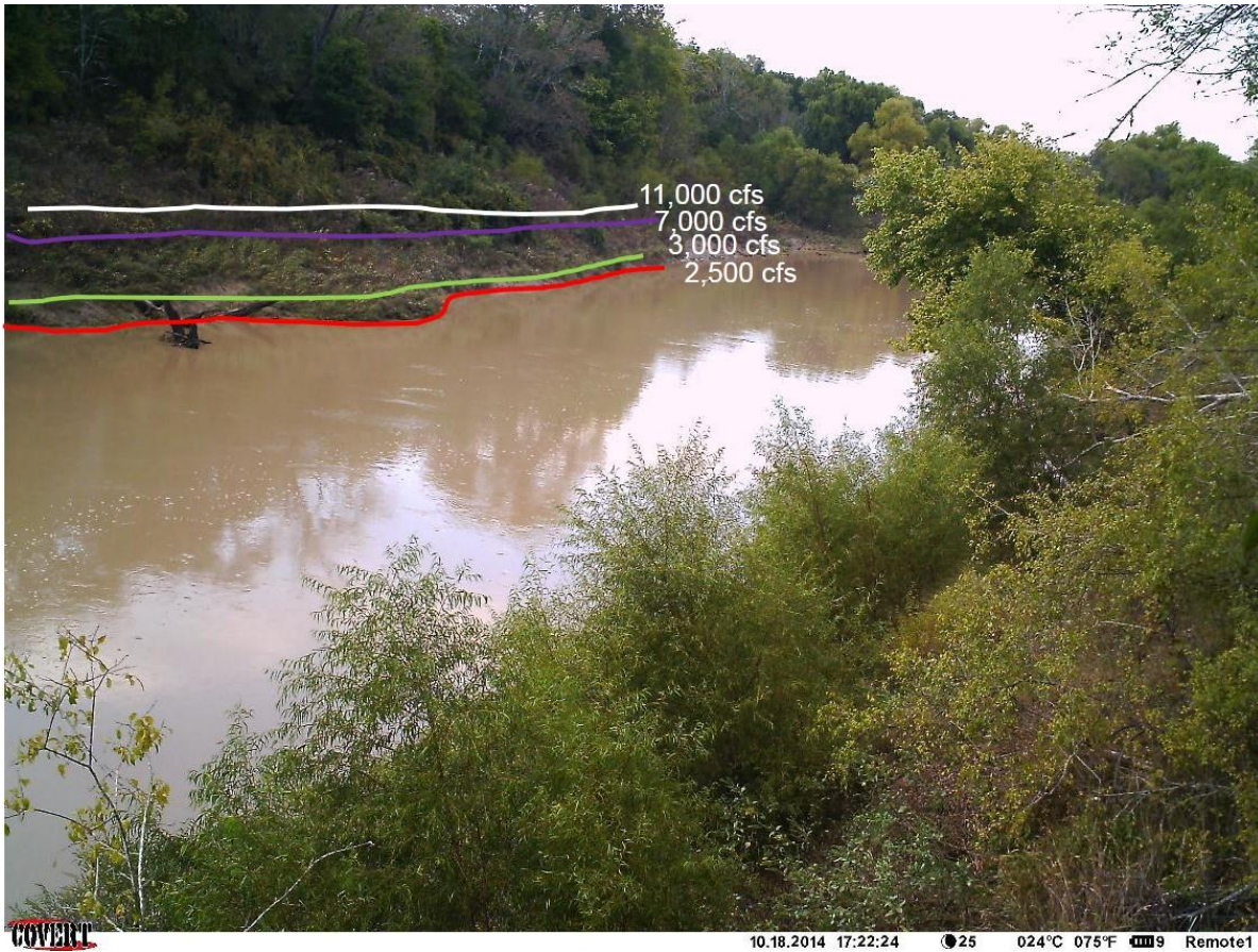
Figure 83. Game camera photograph showing the water line at 1,000 cfs and approximately 11,000 cfs.
