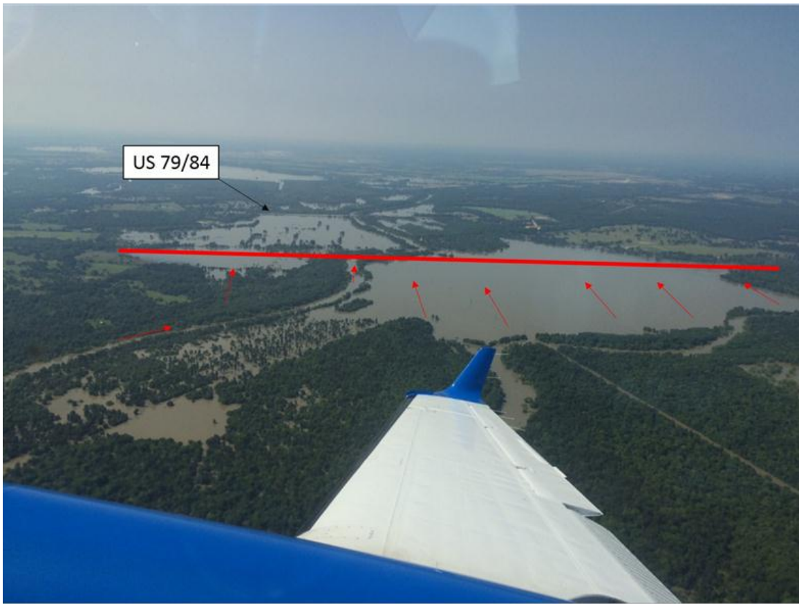
Figure 86. 080295 – Overbank flow condition and velocity direction, at same cross-section. The river reach under the airplane wing is experiencing reverse flow; the reach behind the wing is experiencing transverse flow.
