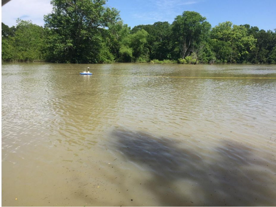
Figure 15. Tethered M9 measuring moving bed at Cross-section 1 at 080295.
