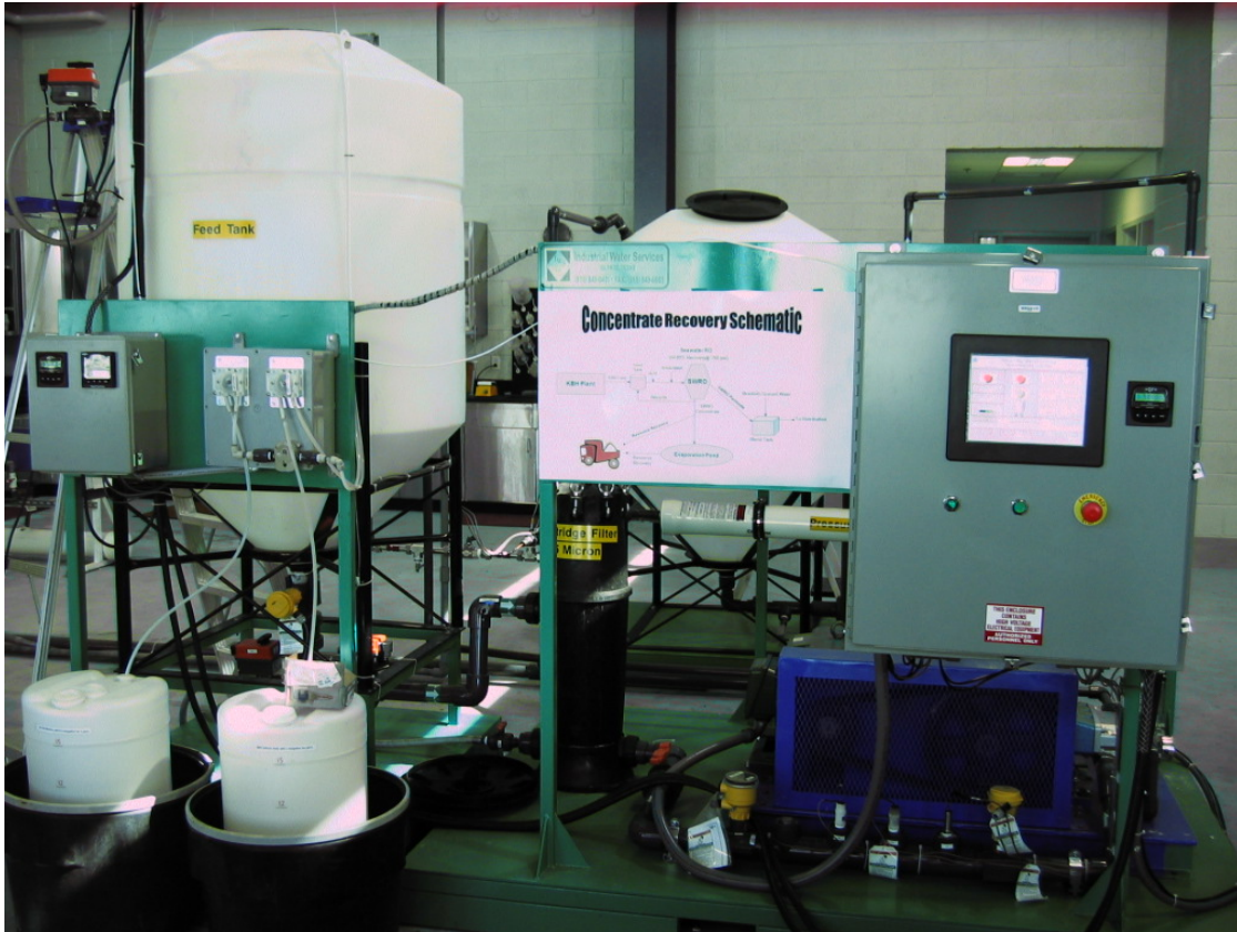
Figure 17. Picture of Fully-Automated Batch Treatment Seawater RO System
