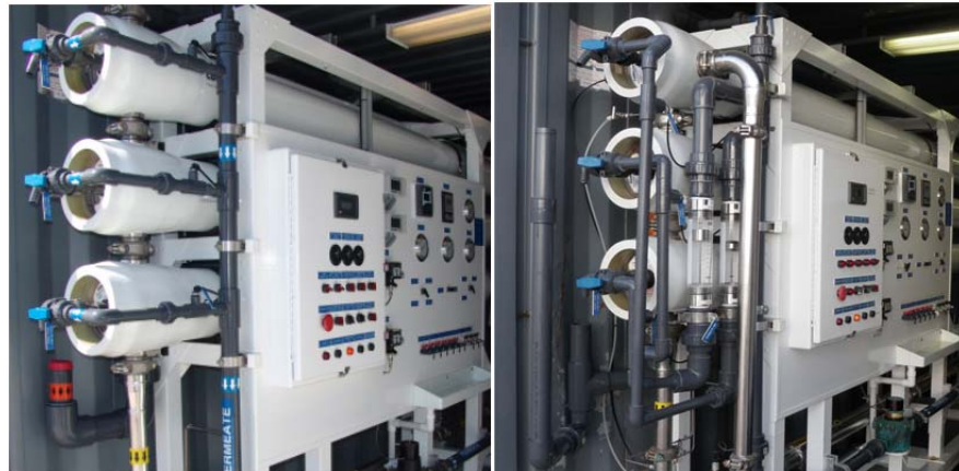
Figure 5. Affordable Desalination Collaboration pilot demonstration unit (Single Stage left view, Two Stage right view).
